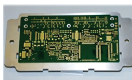
Internal Metalized Heatsink
